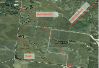
The leak detection system and base station enables Frank and Carole to track and record the hourly, daily and monthly water flows and most importantly detect any water leaks or excessive usage. Frank has programmed the base station's warning system to alert them of excessive flows via a flashing light at the homestead. Warning categories include:
