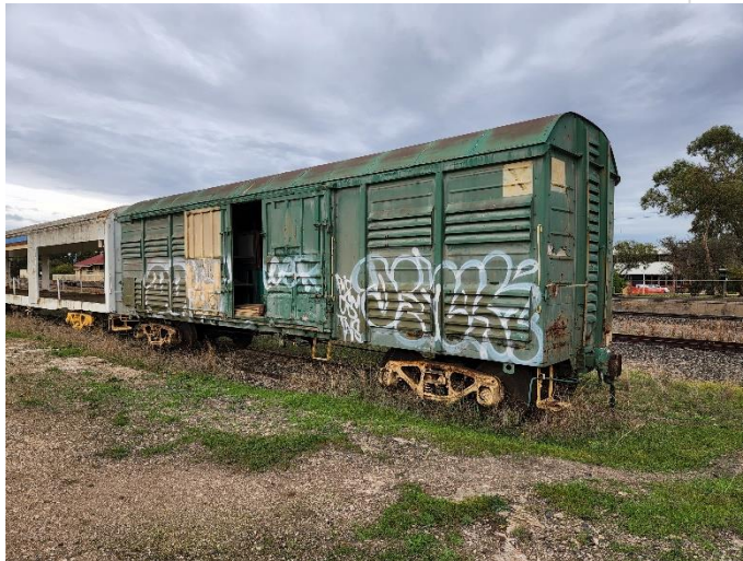
No 6: Green metal clad enclosed carriage, 12.5m long nett
