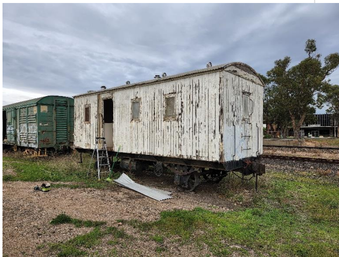
No 7: White timber sided enclosed accommodation carriage. 8m long nett
