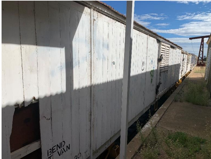
No 2: Timber sided Accident Van No 1, M8213. 13.5m long nett. Contains tools and recovery gear
