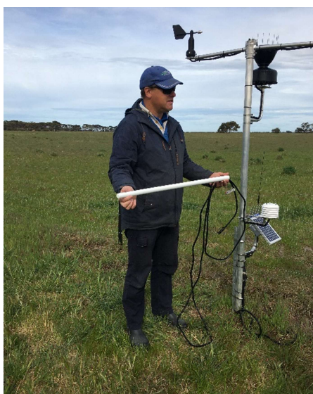
Fig 1. Shane Oster, Alpha Group Consulting installing automated weather station and probe at Elephant Lake, 2020
