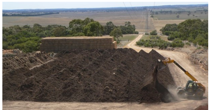
Figure 1. Compost piles being turned to promote microbial activity and stimulating decomposition processes (courtesy Mulbarton Compost).
