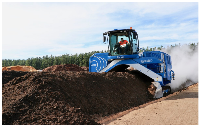
Figure 3. Compost row being turned at Bio Gro Wandilo site with a Windrow Turner (courtesy Bio Gro).
