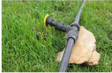
Quick coupling valves or Camlock fittings can be used for quick and easy movement of troughs
