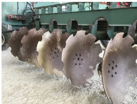
Figure 11a. John Shearer one-way 5GP plough, modified to fit Plozza discs.
