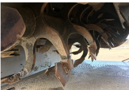
Figure 10a. Triangular shaped spades on curved tines are fixed to a central shaft that rotates at ~90 revs/min 10 .
