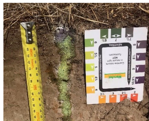
Figure 4. Example soil pit face with pH indicator dye applied. An alkaline surface layer can be seen (purple), overlying acidic soil (bright green) below 3 cm.
