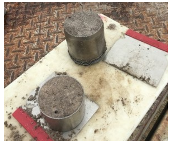
Figure 6. Use a steel ring to extract an intact soil core to determine the bulk density.
