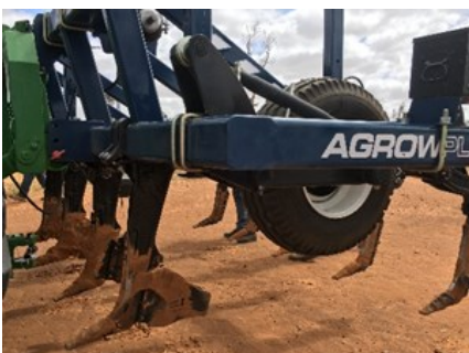
Figure 9a. Example of straight shank tines (AgrowPLOW AP51 Ripper) with inclusion plates fitted.
