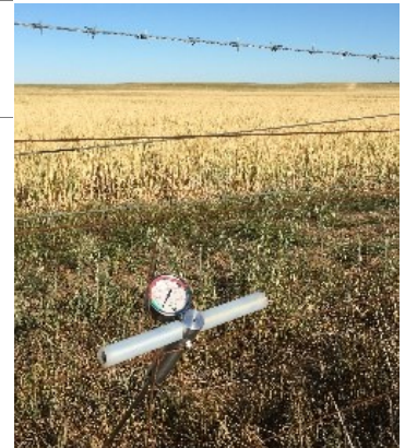
Figure 5. An example of an instrumented cone penetrometer, sourced here .
