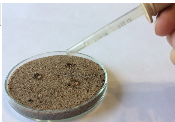
Figure 3. Soil is severely repellent if a droplet of water remains on the surface for longer than 4 minutes.
